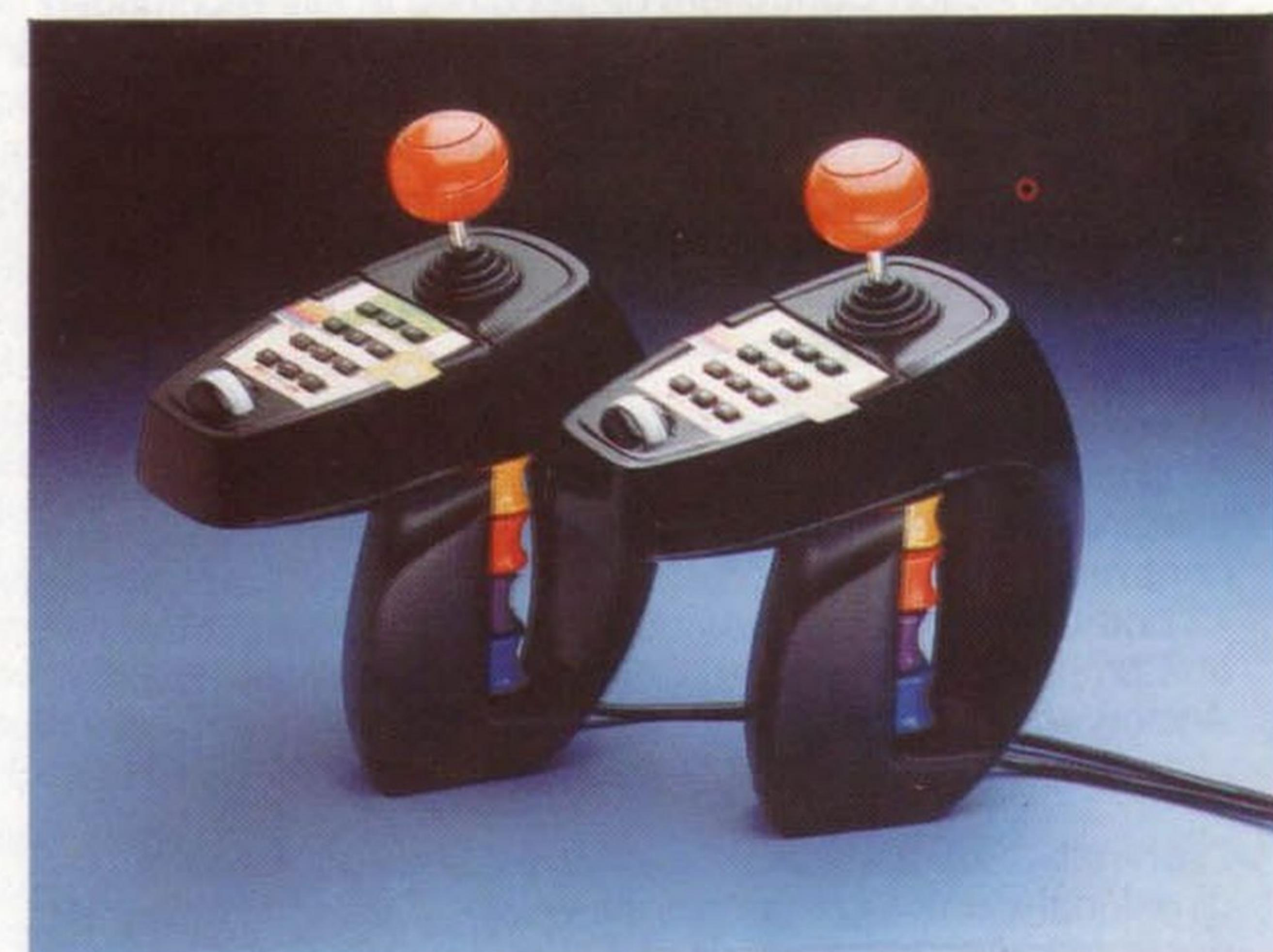
The Super Action Controllers are equipped with a multi-directional joystick, a speed roller, four multiple-use player-select triggers for controlling up to four different objects, a 12 button key pad for greater game-play options, and a customer designed grip for easier handling. The Super Action Controllers will come with the Rocky cartridge.
